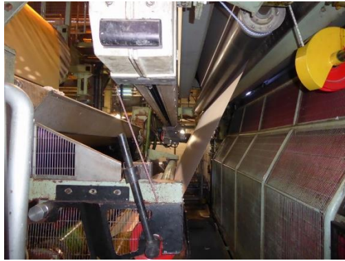
Honeywell web inspection prior to calendar for hole and dirt detection. Machine scanner year 2006 measuring gsm, moisture, profile, opacity.
