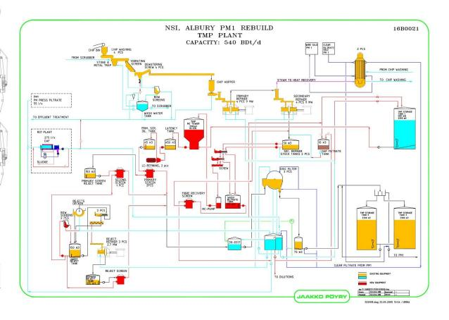
TMP: 540 BDT/day average after the 2005 upgrade. Four main lines with primary and secondary refining. Each 200 BDt/day
